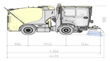
Length with standard brush 4,300 mm Length with 3rd brush 5,020 mm Width 1,150 mm 1,990 mm Height Sweeping width standard brush 2,300 mm Sweeping width with 3rd brush 2,600 mm Turning circle 6,650 mm Turning circle 'kerb to kerb' 6,050 mm
